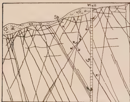
FIG. 33.—Diagram showing the source of well and spring water in fractured rock. (Modified after H. E. Gregory.)
